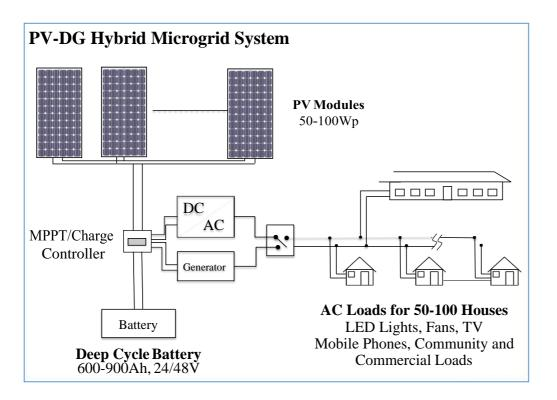
Generator AC power output can be directly connected to AC loads. A transfer switch is needed to prevent generator power from feeding backwards in the inverter. The transfer switch can be electronically operated or a manual change over switch. The generator can also be used to recharge the batteries.
